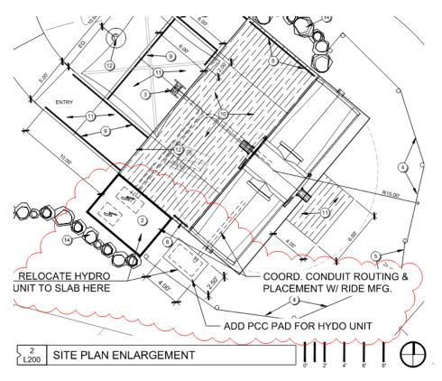
**Sheet A100.** Hydraulic unit for ride to be located outside of shed due to clearance requirements.
